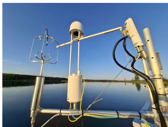
Fig.1. Floating platform equipped for greenhouse gas flux measurements using the eddy covariance method in the Kuibyshev Reservoir ( https://kpfu.ru/ecology/karbon-povolzhe , photo: V.E. Prokhorov).
