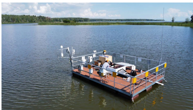
Fig.1. Floating platform equipped for greenhouse gas flux measurements using the eddy covariance method in the Kuibyshev Reservoir ( https://kpfu.ru/ecology/karbon-povolzhe , photo: V.E. Prokhorov).
